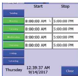
Figure 7-12: Input field for determining heating phases Adjust here when the hygieniser should heat (dates and times).
